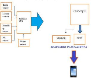
Figure 1.Proposed Automation of Irrigation System.
